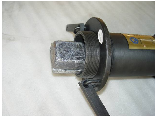
push the alloy to the bottom
