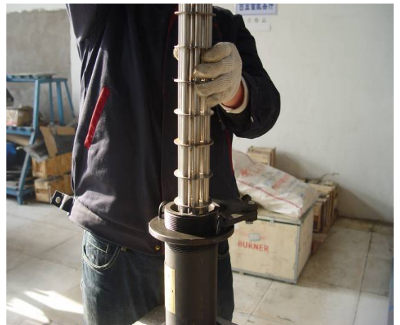
insert the heating element to the tube when all conductor melt
