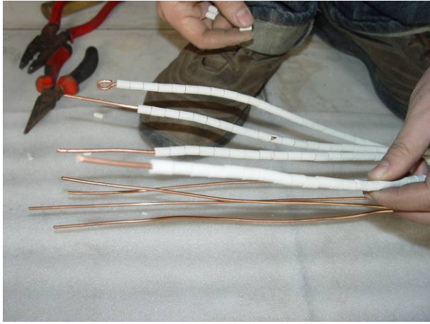
No ceramic bead in the zero line
