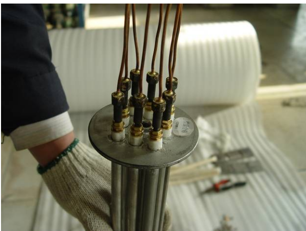
identify two-phase of the four heating cores
