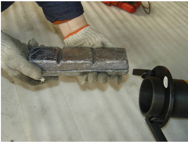
Put two pieces of heat conductor together into tube
