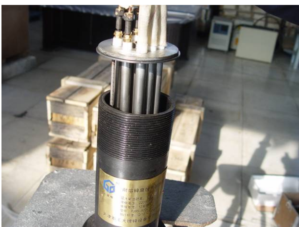
Pre-heat the heating element in the tube for a moment
