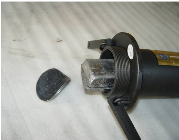
Make sure no conductor left
