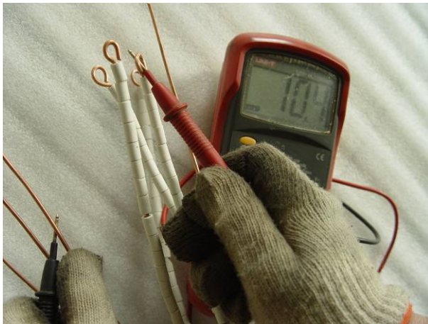
Check whether there is short or open circuit in each heating core
